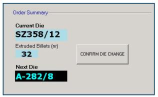
**4.** With the **die recipe database**, each die copy has its own unique recipe. The operator simply selects the die copy for each order to automatically load the optimal recipe values into the system.
