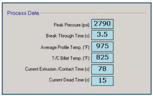
3. **Critical process data** is displayed for each billet on the operator console and more extensive data is saved for each billet and order in the advanced system reports.
