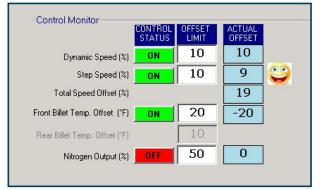
2. The closed loop control system continuously and automatically adjusts the press speed and billet feed temperatures to optimize breakthrough times, maximize pressure, and maintain optimal profile temperatures at the exit of the press.
